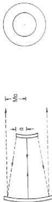
Figure 14.33 A positive-branch ( $g_1 g_2 > 1$ ) confocal unstable resonator. The near-field output is a collimated, annular beam.
