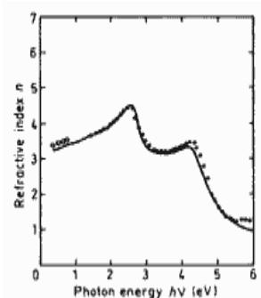
**Refractive index  $n$  versus photon energy for  $x=0.47$ , 300 K.**
