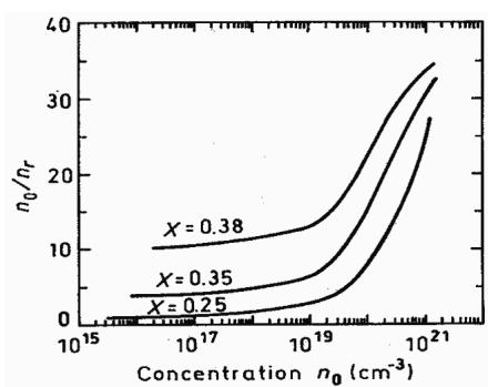
**Ratio of the total carrier concentration to the carrier concentration in  $\Gamma$ -valley as a function of equilibrium carrier concentration at 300K (Zarem et al. [1989]).**
