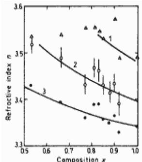
**Refractive index  $n$  versus alloy composition  $x$  at different photon energies**
