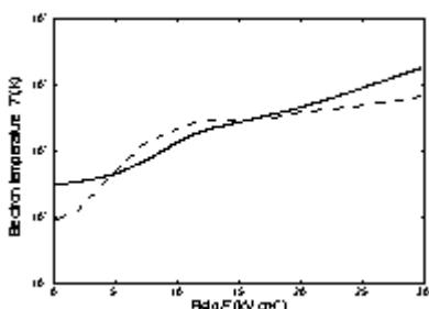
**Electron temperature versus electric field for 77 K and 300 K.**
