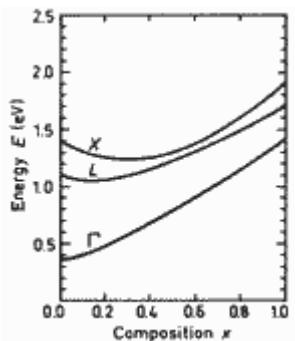
**Ga<sub>x</sub>In<sub>1-x</sub>As.** Energy gap  $E_g$  Energy separations between  $\Gamma$ - ,X-, and L-conduction band minima and top of the valence band vs. composition parameter  $x$ .
