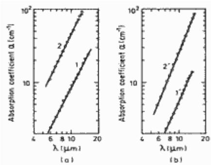
**Free carrier absorption coefficient versus wavelength.**
