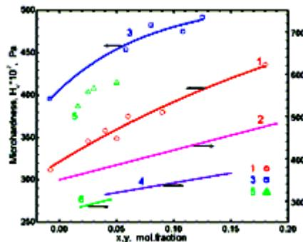
**Micro hardness (Hv) and energy gap values  $E_g$  vs composition of three alloy systems:**
