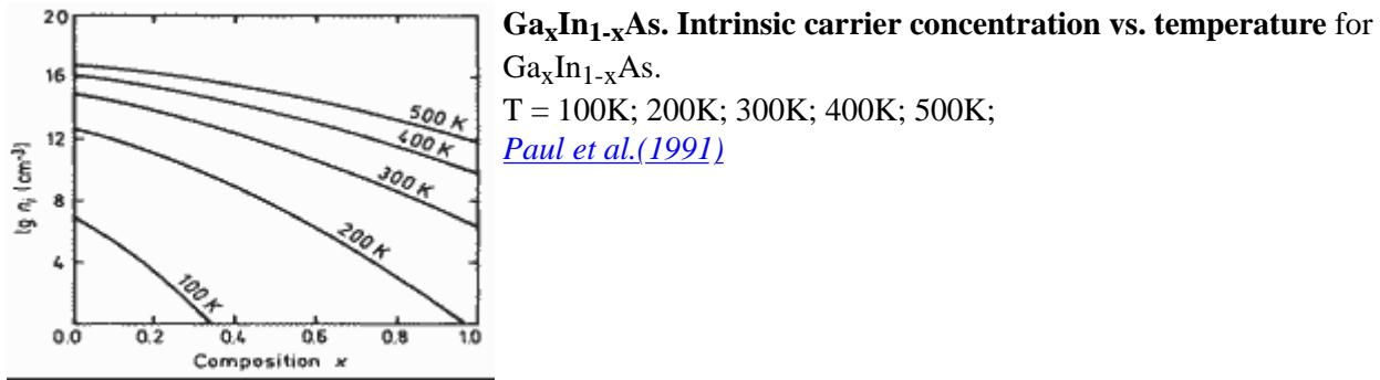
$$n_i = 6.3 \times 10^{11} \text{ cm}^{-3} \text{ for Ga}_{0.47}\text{In}_{0.53}\text{As at 300K}$$
