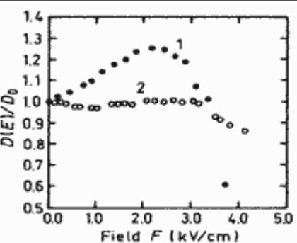
**The field dependences of normalized longitudinal diffusion coefficient.**
