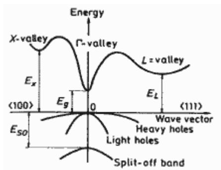
**Band structure Al<sub>x</sub>Ga<sub>1-x</sub> for x<0.41-0.45. Important minima of the conduction band and maxima of the valence band**
