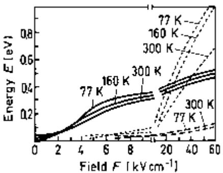
**Mean energy  $E$  in  $\Gamma$ ,  $L$ , and  $X$  valleys as a function of electric field  $F$  at 77, 160, and 300 K,  $N_d=0$**
