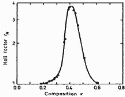
**Hall factor versus alloy composition x for n-type  $\text{Al}_x\text{Ga}_{1-x}\text{As}$  T=300 K**
