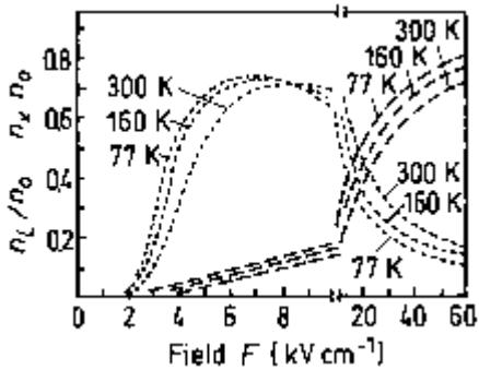
**Fraction of electrons in  $L$  and  $X$  valleys.  $n_L$  and  $n_X$  as a function of electric field  $F$  at 77, 160, and 300 K,  $N_d=0$**
