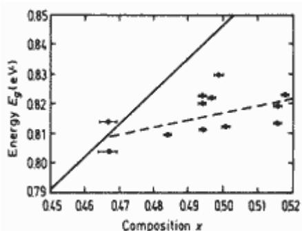
**Ga<sub>x</sub>In<sub>1-x</sub>As.** Energy band gap  $E_g$  of unstrained (solid line) and strained (dashed line and experimental points) vs. composition parameter  $x$ .
