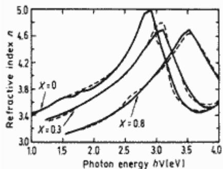
**Refractive index  $n$  versus photon energy for three values of  $x$ .**
