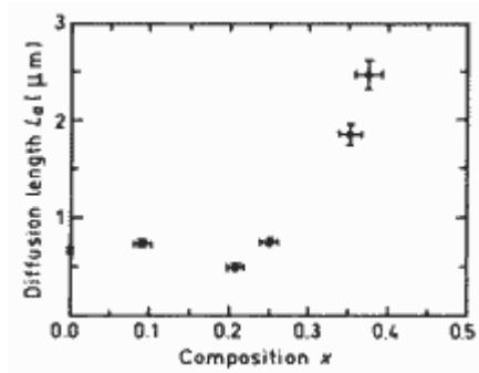
**Ambipolar diffusion length at a carrier density of  $10^{17}\text{--}10^{18} \text{ cm}^{-3}$  versus  $x$ . T= 300K.**
