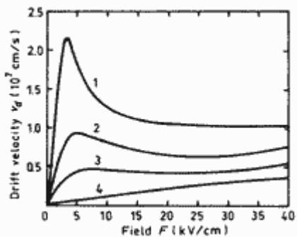
**Field dependences of the electron drift velocity for different values of x.**
