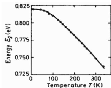
**Ga<sub>0.47</sub>In<sub>0.53</sub>As. Energy gap E<sub>g</sub> of vs. temperature**
