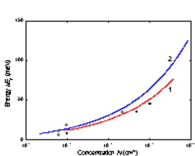
Energy gap narrowing versus donor (curve 1 and experimental points) and acceptor (curve 2) doping density, T = 300 K.
