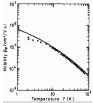
**Hole mobility in 2D-hole gas versus temperature.**
