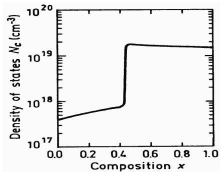
**Effective density of states in the conduction band versus x.**
