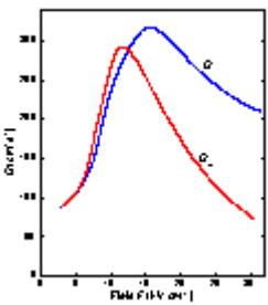
**Longitudinal ( $D \parallel F$ ) and transverse ( $D \perp F$ ) electron diffusion coefficients at 300 K.**
