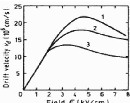
Experimental field dependences dependences of electron velocity.
