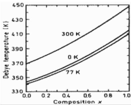
**Debye temperature as a function of x for three different temperatures.**
