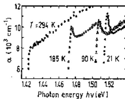
Intrinsic absorption coefficient near the intrinsic absorption edge for different temperatures. ([Sturge \[1962\]](#)).
