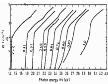
**Intrinsic absorption coefficient near the intrinsic absorption edge for different values of  $x$ . 300 K.**
