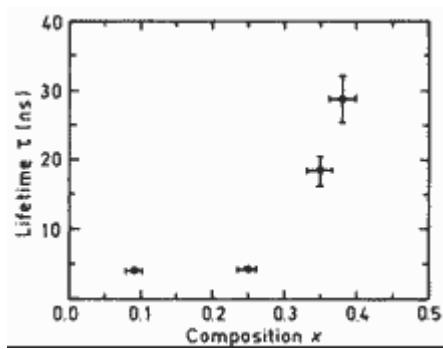
**Carrier lifetimes at carrier density of  $\sim 3 \cdot 10^{18} \text{ cm}^{-3}$  (high injection level) versus versus  $x$ . T= 300K.**
