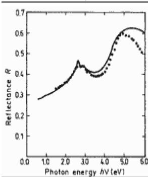
**Normal incidence reflectivityversus photon energy for  $x=0.47$ , 300 K.**
