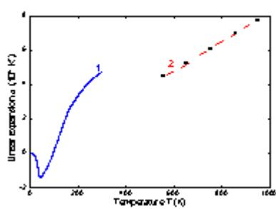
**Temperature dependence of linear expansion coefficient  $\alpha$ .**
