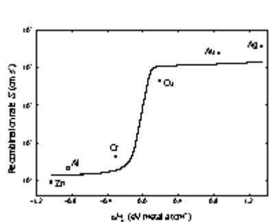
**Surface recombination velocity versus the heat of reaction per atom of each metal phosphide  $\Delta H_R$**
