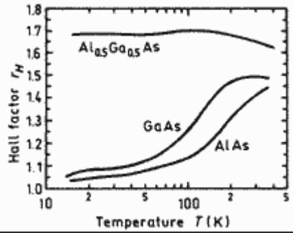
**Hall factor versus temperature x for p-type GaAs, AlAs and  $\text{Al}_{0.5}\text{Ga}_{0.5}\text{As}$ .**
