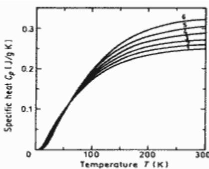
**Ga<sub>x</sub>In<sub>1-x</sub>As. Specific heat at constant pressure vs. temperature for different concentrations x.**
