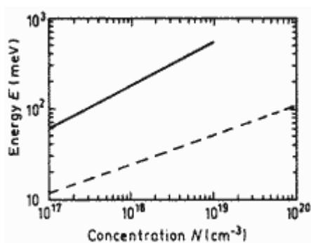
**Ga<sub>0.47</sub>In<sub>0.53</sub>As. Energy gap narrowing E<sub>g</sub> vs. donor (solid line) and acceptor (dashed line) doping density**
