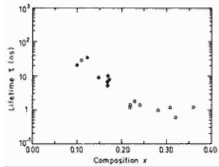
**Hole lifetime versus  $x$  for n- $\text{Al}_x\text{Ga}_{1-x}\text{As}$**
