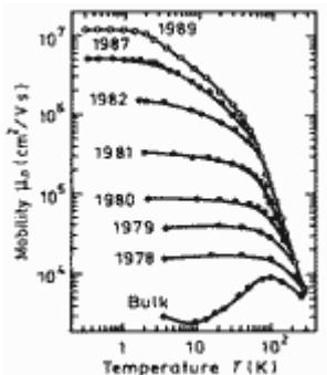
Temperature dependences of the electron Hall mobility in the modulation-doped two-dimensional gas.
