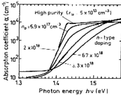
**Intrinsic absorption edge at 297 K at different doping levels. *n*-type doping**
