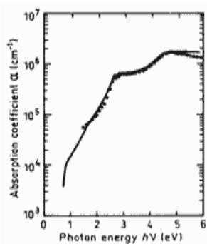
**The absorption coefficient versus photon energy for  $x=0.47, 300 \text{ K}$ .**
