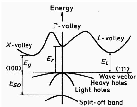
**Band structure  $\text{Al}_x\text{Ga}_{1-x}$  for  $x > 0.45$ . Important minima of the conduction band and maxima of the valence band**
