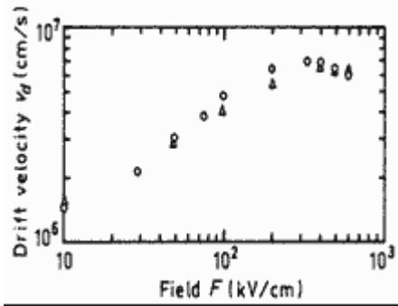
Field dependence of hole drift velocity. Monte-Carlo calculations.
