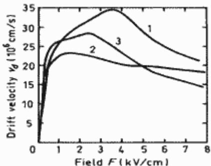
Experimental field dependences dependences of electron velocity.
