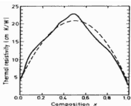
**Ga<sub>x</sub>In<sub>1-x</sub>As. Thermal resistivity vs. composition parameter x**
