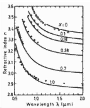
**Refractive index  $n$  versus wavelength for different values of  $x$ . 300 K.**
