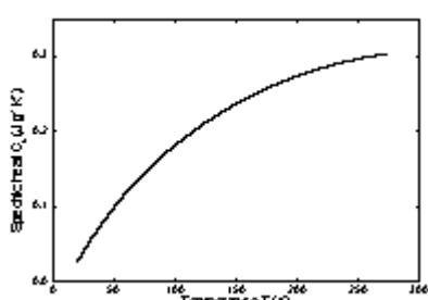
**Temperature dependence of specific heat at constant pressure**
