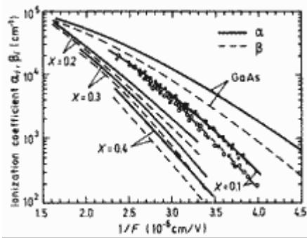
Fits to experimental values of electron and hole ionization coefficients for  $\text{Al}_x\text{Ga}_{1-x}\text{As}$  with  $x=0.1\div0.4$ .  $T=300$  K.
