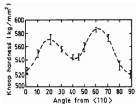
Knoop microhardness anisotropy on the {100} plane for Ga<sub>0.47</sub>In<sub>0.53</sub>As.
