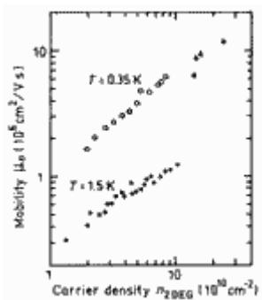
Dependences of electron mobility versus surface carrier density 2D electron gas in the modulation-doped two-dimensional gas.
