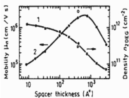
Dependences of surface electron density (Curve 1) and mobility (Curve 2) versus undoped spacer thickness.  $T=4 \text{ K}$ .
