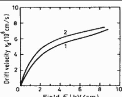
Experimental field dependences of hole velocity for two-dimensional hole gas. Single heterointerface samples.  $x=0.5$ .  $T=77\text{ K}$ .
