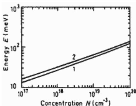
Energy gap narrowing versus donor (curve 1) and acceptor (curve 2) doping density for AlAs ( $x=1$ ).
