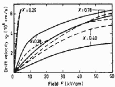
**Field dependences of the electron drift velocity for different values of x.**
