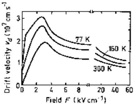
Field dependences of the electron drift velocity at different
