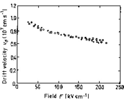
Field dependences of the electron drift velocity for high electric fields,
