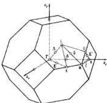
Brillouin zone of the face centered cubic lattice, the Bravais lattice of the diamond and zincblende structures.
