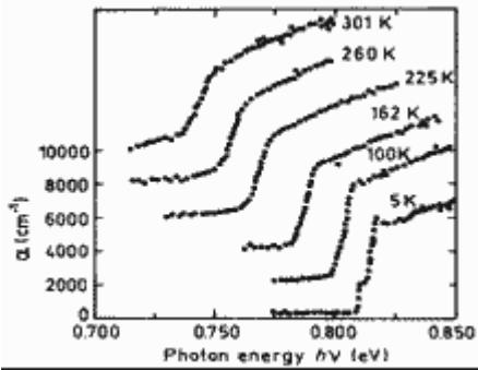
**The absorption coefficient versus photon energy at different temperatures for  $x=0.47$ .**
