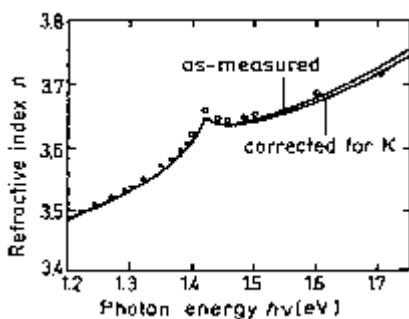
Refractive index  $n$  versus photon energy for a high-purity GaAs. ( $n_0 \sim 5 \cdot 10^{13} \text{ cm}^{-3}$ ).
