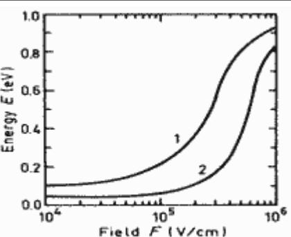
**Average electron energy as a function of electric field.  $T=300$  K.**
