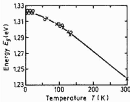
**Ga<sub>0.87</sub>In<sub>0.13</sub>As. Energy gap E<sub>g</sub> of vs. temperature**
