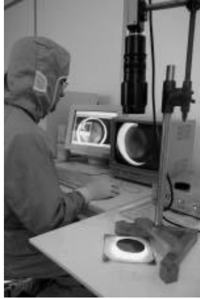
Figure 8. IR-camera inspection set-up.
