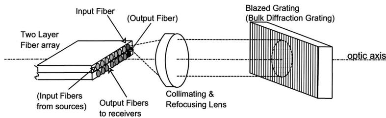
Fig. 4 The structure of dual deck WDM device for bidirectional transmission.
