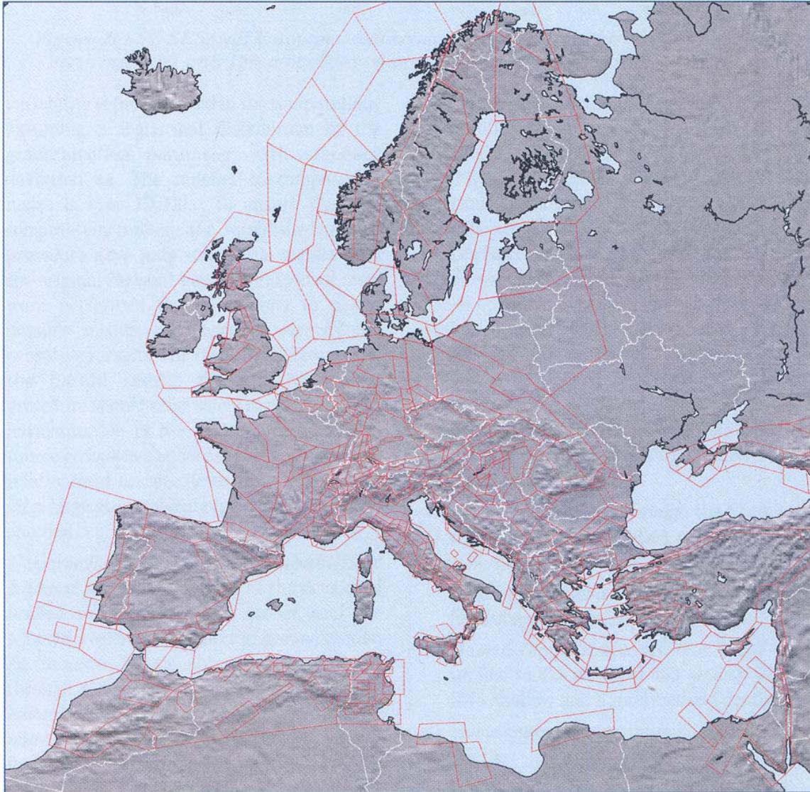
Figure 6.1. The unified source model with its 463 seismic sources *for the european-mediterranean region [20,21].*
