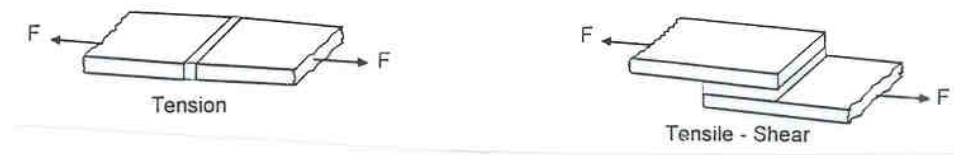
Fig. 9: Adhesive joint design. Left figure not suitable. Right figure typical adhesive joint design.
