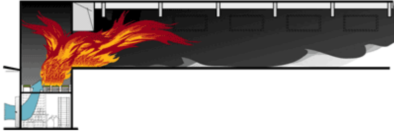
Figure 9 d. The flames filled the entire door opening and ignited the floor.
