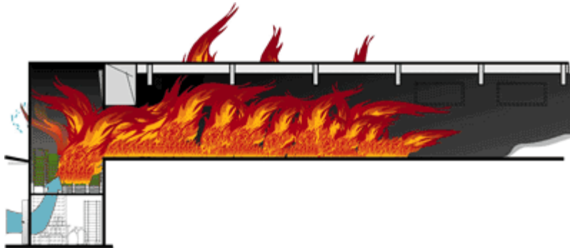
Figure 9 e. The floor was the main contribution to the vigorous fire; flames shot out from the side windows.
